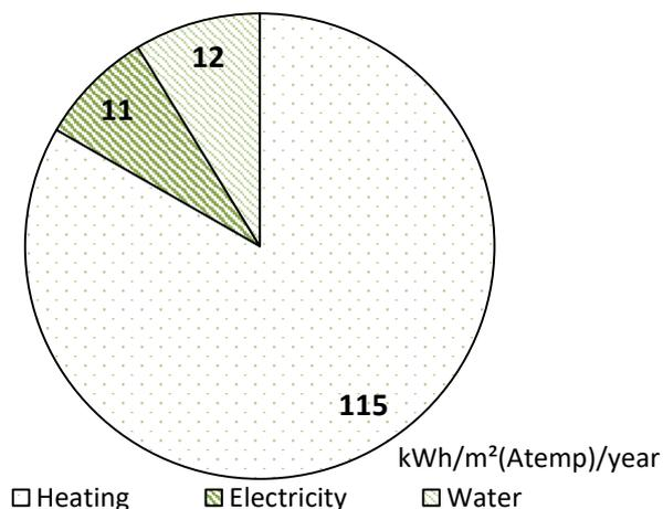
Figure 3. Energy demand before renovation based on statistical data from 5-year period (2009-2013) measured by LKF (Heating and Water together  $\pm 13$  kWh/m<sup>2</sup>/year).
