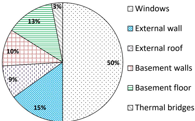
Figure 5. Heat losses from transmission for the pilot dwellings.
