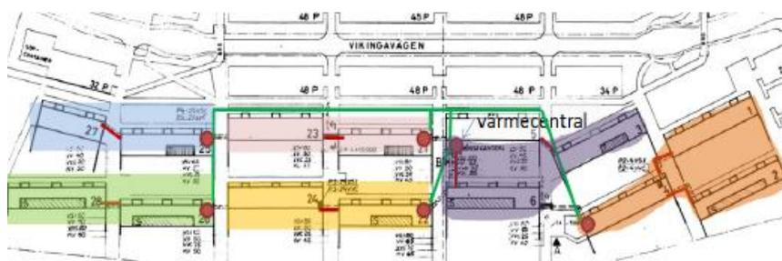
Figure 6. District heating network retrofit with 6 smaller substations.
